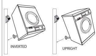
You will need to pack at the bottom spacers by the same thickness as the batten to keep the dryer upright and level.
