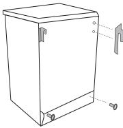
When locating the mounting brackets onto the dryer back panel, you may notice only one screw hole. If this is the case, you will need to take the other self-tapping screws to push and pierce the dryer back panel. (this will locate the hole beneath the back panel). Continue to turn the self-tapping screws until tightens. Once done, in the same manner fit the spacers to the back of the dryer.
