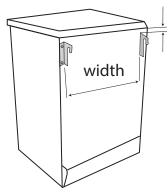
Note the measurements from the top of the dryer to the top of the dryer bracket and the distance between the dryer brackets etc.
